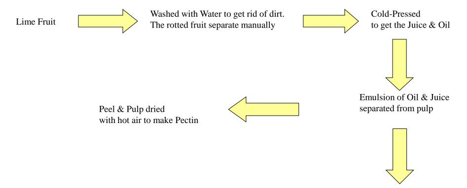
Emulsion containing Oil & Juice centrifuged to separate Oil from the Juice
